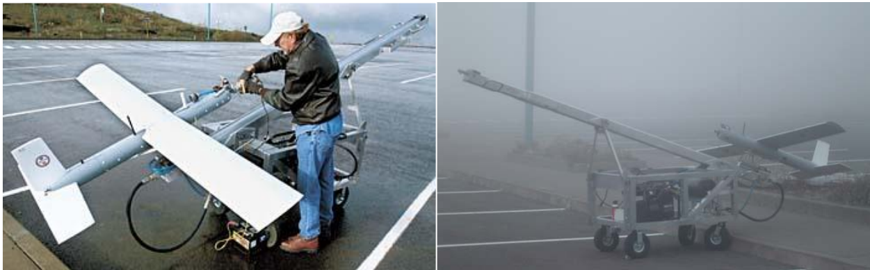
Figure 3. Silver Fox mounted on the pneumatic catapult in the parking lot where it was launched and recovered
