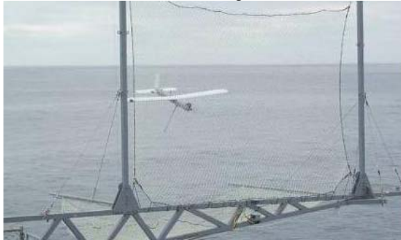
Figure 7. Initial manual net capture tests on the Lockheed Martin Sea Slice vessel in 2004.
