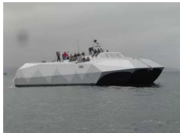
Figure 9. The US Navy's experimental hull littoral combat vessel "Stiletto" used as a platform for autonomous vehicles.
