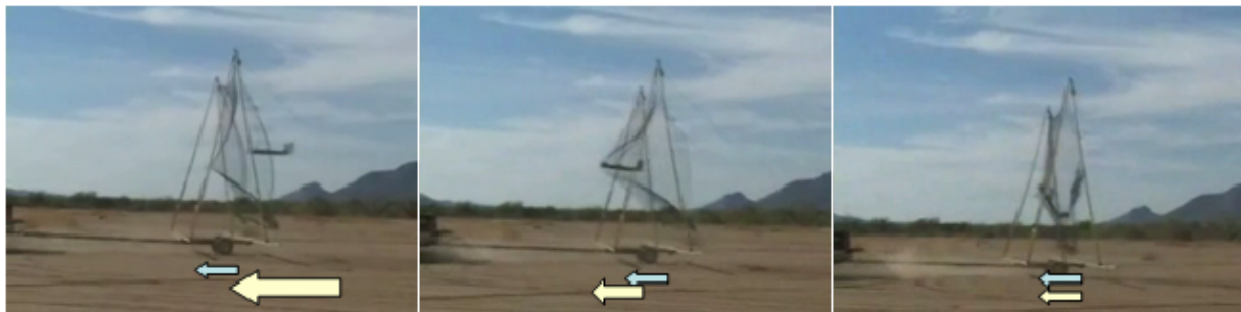
Figure 6. Sequence of photographs showing the capture of a Silver Fox UAV into a moving net travelling in the same direction. The arrows indicate the relative speed of the net and UAV.
