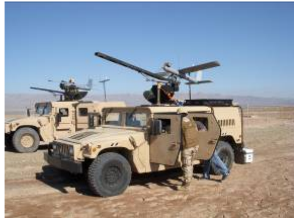
Figure 1. Silver Fox UAS consisting of three UAVs, launcher, ground control station (iGCS) – package fits in standard HUMVEE.
