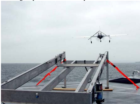
Figure 11. Manta UAV with hyperspectral imager being launched during the Howler Exercise at sea from the deck of the Stiletto
